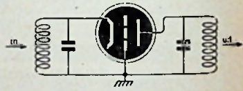
Fig. 4 Zg. rooster basis-schakeling
